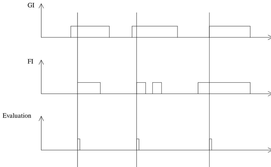
The evaluation is enabled once by GI. The next single evaluation is initiated by resetting and then setting GI again. Only the rising edge is evaluated. The sequence of FI and GI is irrelevant.
