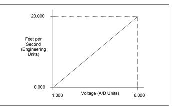
For this example, 1.0V to 6.0V is the normal voltage range, but the module will attempt to scale the inputs for a voltage that lies outside the range. If a voltage of 10.0V were input to the channel, the module would return a scaled channel value of 36.000. The application should use alarms or take other precautions for scaled inputs that are outside the acceptable range or invalid.
