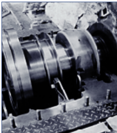
Mounting example PR 6426 transducer for measurement of differential expansion
