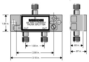
Schneider Electric MA-0186-100 (PV:01) Splitter dimensions:
