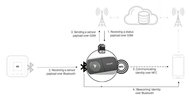
**Figure 1. The iotspot module and its six functions explained.** The iotspot module and the three communication components; GSM, Bluetooth and NFC, are depicted in black, while the ancillary devices and infrastructure are shown in light grey.
