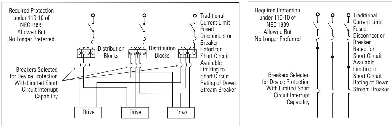
Use class CC, J, L, or R fuses, with current rating as indicated in the table below. The following fuse examples and Allen-Bradley circuit breakers are recommended for use with integrated axis modules (2094-*xCxx-Mxx-S*) when the Line Interface Module (LIM) is not used.
