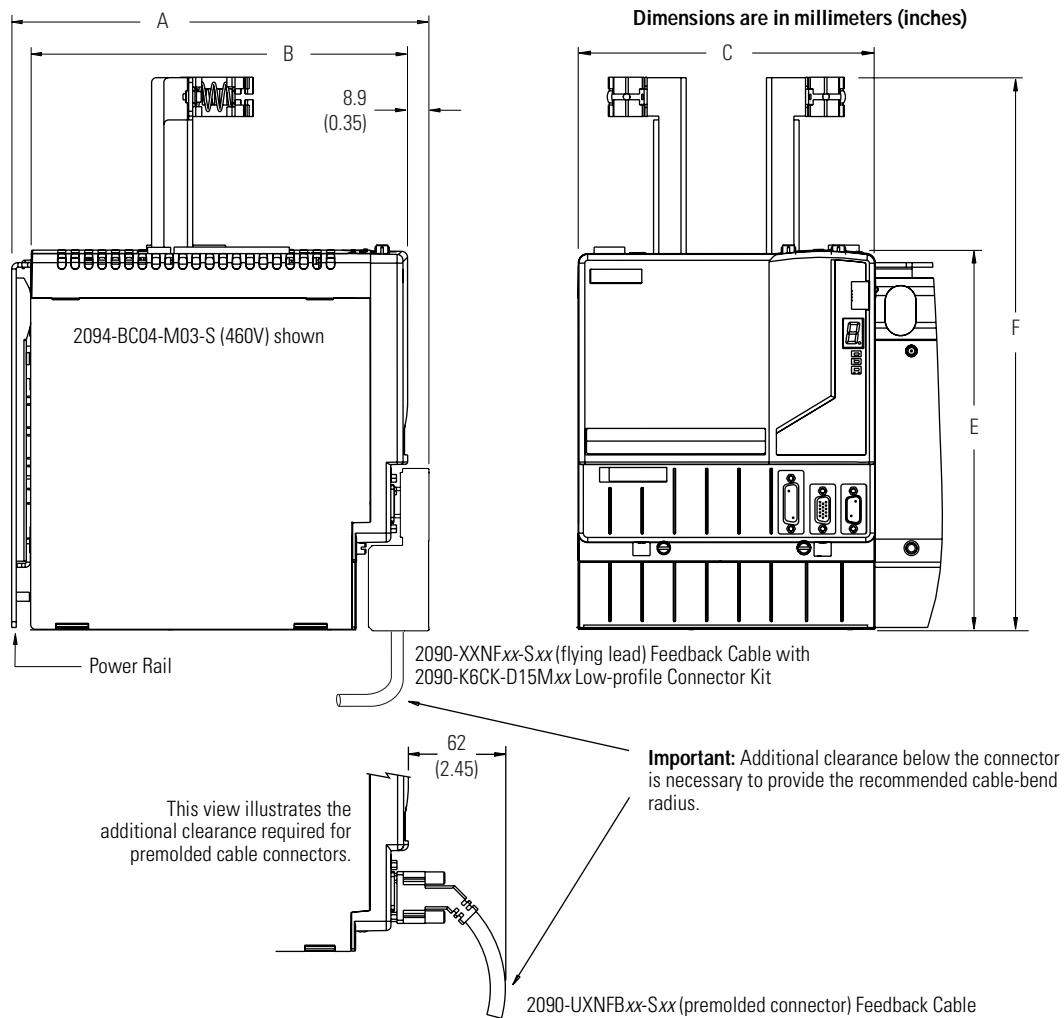
Modules are shown mounted to the power rail and the dimensions reflect that in the depth of the module.
