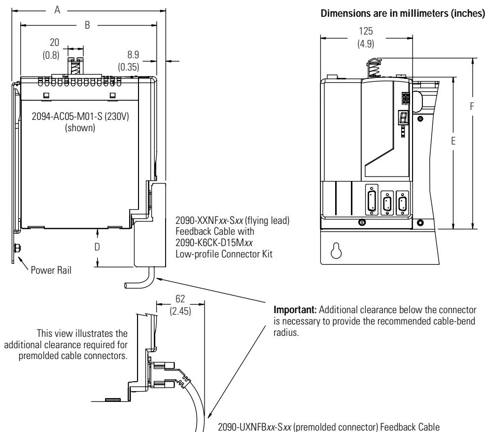
Modules are shown mounted to the power rail and the dimensions reflect that in the depth of the module.
